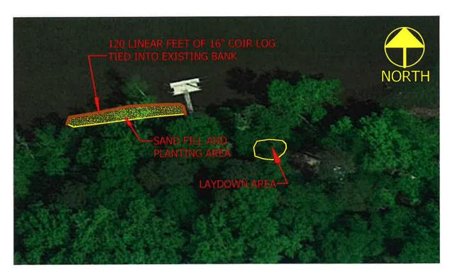
COIR LOG TOE STAKED IN PLACE NO MORE THAN 12 FEET CHANNELWARD OF EXISTING EROSION SCARP. SAND FILL DELIVERED TO SHORELINE VIA A TEMPORARY PLYWOOD FLUME OR CONVEYOR FROM TOP OF BANK. TREE THINNING TO OPEN UP SUNLIGHT TO INCLUDE LIMBING OF TREES AND SAPLINGS.
